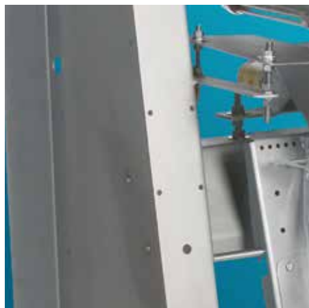
The AccuFill® weigh/bagging system's open-frame design leaves no place for debris to hide or water to pool.
